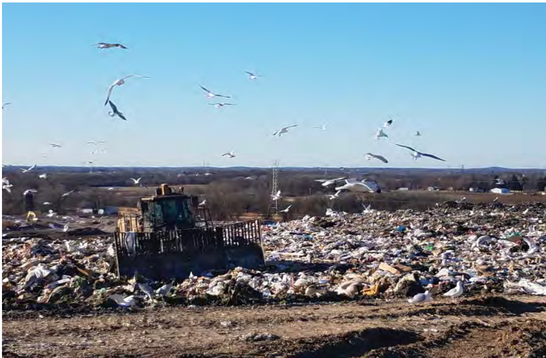
Compactor working in Phase 7 South, against Phase 7 North, nearly same elevation
