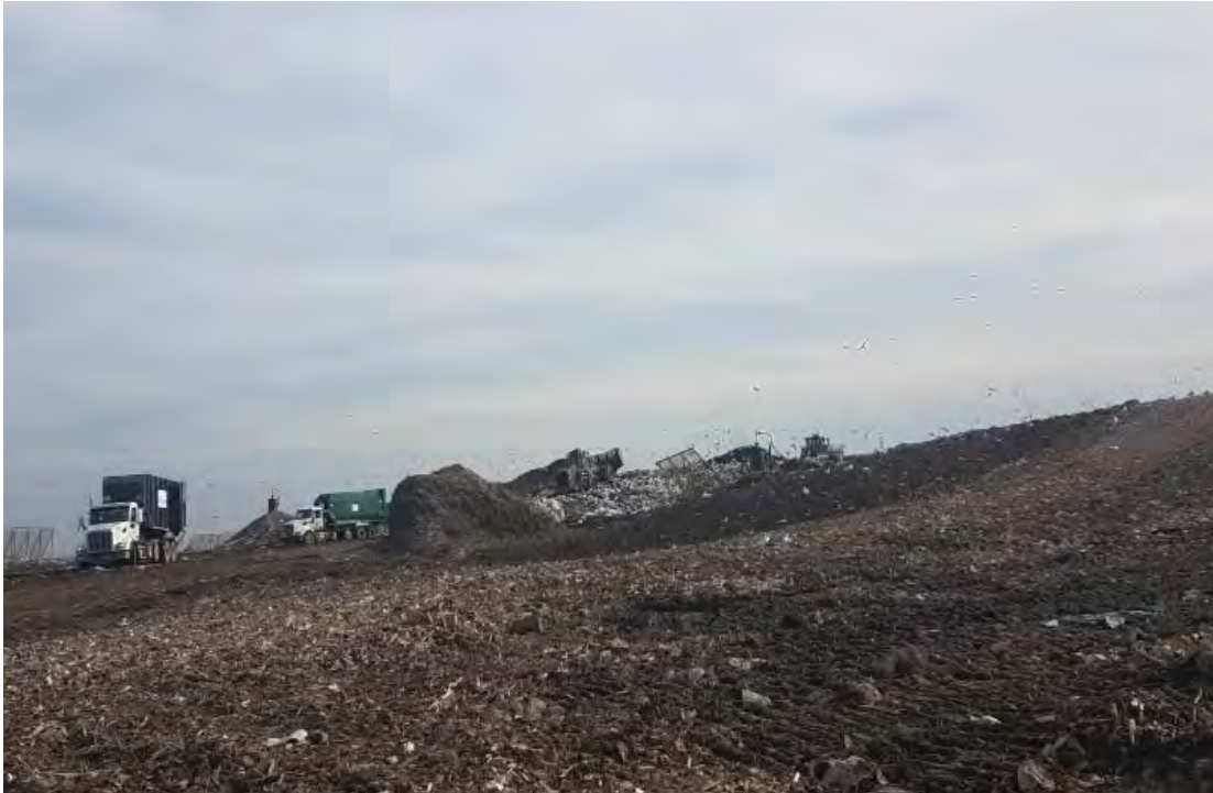
Working face filling in adjacent to yesterdays waste placement, wind protected by previous lift
