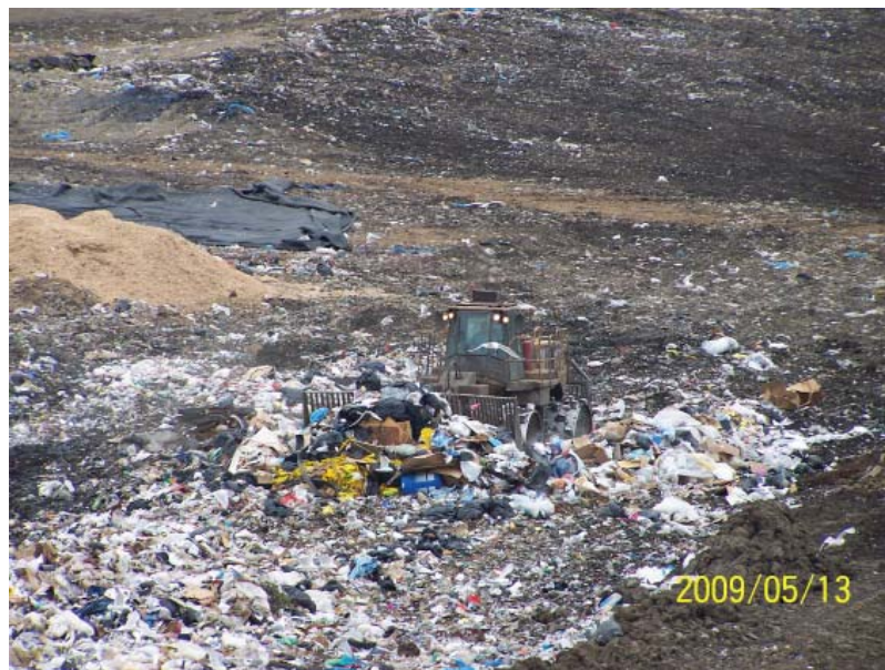
Compactor moving waste into place for compaction
